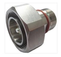
Product Classification **Product Type** Adapter **General Specifications Body Style** Straight **Inner Contact Plating** Silver Interface 4.1-9.5 DIN Female Interface 2 7-16 DIN Male **Mounting Angle** Straight **Outer Contact Plating** Trimetal Pressurizable No Dimensions Length 35 mm | 1.378 in Diameter 34.6 mm | 1.362 in
