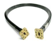
FlexTwist® Flexible Twist for WR42, 17.7–2 6.5 GHz, with interface types PBR220 and PBR220, 900 mm
